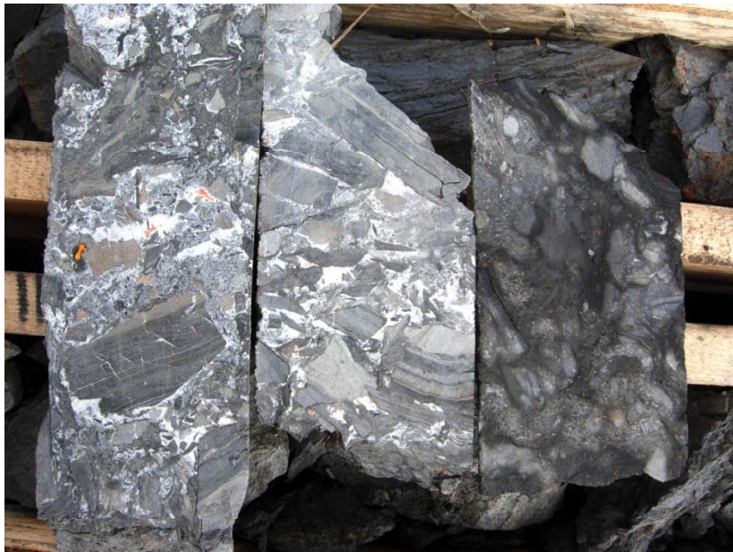
Photos of drill core from Rackla gold district, showing decalcified Proterozoic limestone with disseminated orpiment. Typical grades for this type of rock are 10-30 ppm Au
