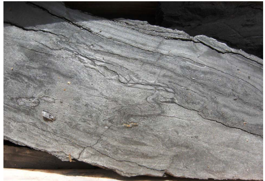
Photos of drill core from Rackla gold district, showing decalcified Proterozoic limestone with disseminated orpiment. Typical grades for this type of rock are 10-30 ppm Au
