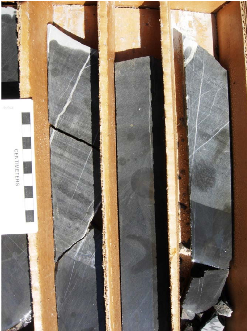
Typical drill core in a Carlin-type carbonate-rock hosted gold deposit: subtle to boring "No-see-um gold"
