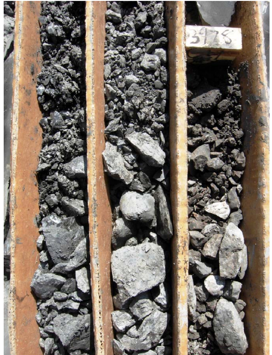
Typical drill core in a Carlin-type carbonate-rock hosted gold deposit: subtle to boring "No-see-um gold"
